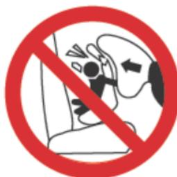
**WARNING:** DO NOT place a child restraint in the front seat of a vehicle with a passenger air bag unless *the air bag is turned off*. DEATH or SERIOUS INJURY can occur. The back seat is the safest.
