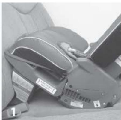
Restraint bottom and base are both flat on the vehicle seat with front of restraint against the back of that vehicle seat. (Fig. 1)
