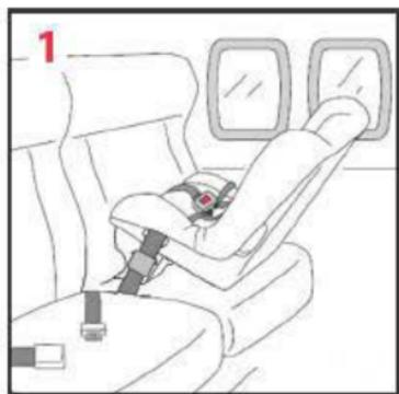
*This restraint is FAA certified for use in an aircraft only as a harnessed restraint. This restraint is NOT certified for use in an aircraft as a belt-positioning booster.*
