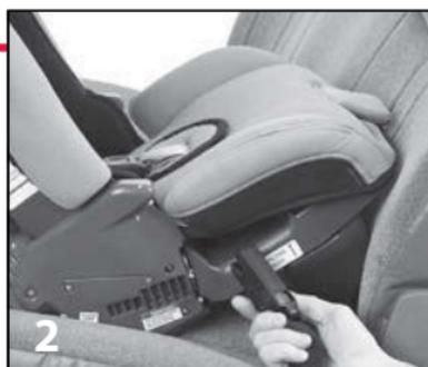
LATCH connector will 'click' to confirm attachment to anchor.
