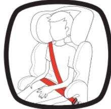
6. Make sure the vehicle seat belt is not twisted and lays flat across child's lap, torso and shoulder.
