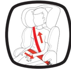
**IMPORTANT:** The Vehicle Shoulder Belt **MUST** route completely through the RED shoulder belt guide and not fall off the child's shoulder.
