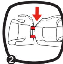
2. Attach the backrest hooks to seat mounting points.
