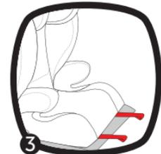
**NOTE:** Even with UAS connectors properly attached and adjusted, child seat will still have movement against the vehicle seat back and bottom.
