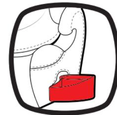
Swivel inward to the recessed and locked position when not in use.
