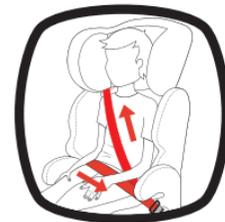
**IMPORTANT:** The vehicle shoulder belt **MUST** route completely through the **RED** shoulder belt guide and not fall off the child's shoulder.
