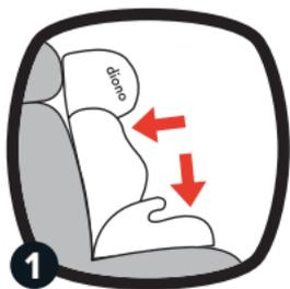
2. Push seat bottom and backrest of booster seat down and back into vehicle seat until there is secure positioning with the booster seat and vehicle seat bottom and vehicle seat back.
