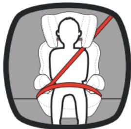
Use **ONLY** the vehicle lap and shoulder belt system when restraining the child in this child restraint. **DO NOT use a lap belt only!**
