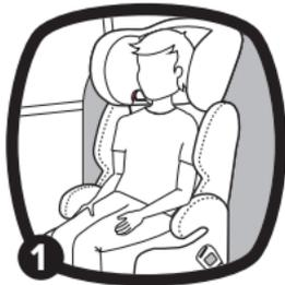
2. **Adjust head support to proper height:** The shoulder belt guide should be slightly above the child's shoulders (at least 2.5 cm).
