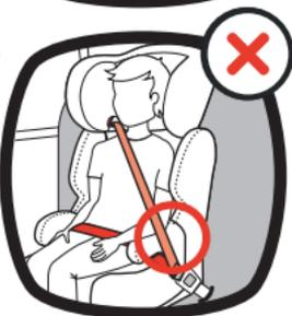
**IMPORTANT:DO NOT** position the vehicle shoulder belt over the armrest. It **MUST** pass through the lower belt guide closest to the vehicle buckle. **ALWAYS** make sure the vehicle seat belt can properly retract before each use.
